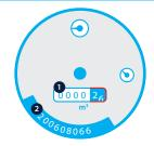
When you send us a meter reading, always exclude any numbers in red. Meters come in all shapes and sizes, this picture shows where you can typically find the reading and the serial number.
